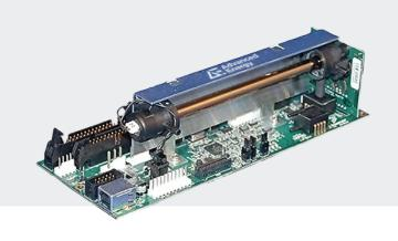
The Andros® 6511 OEM gas module achieves high reliability through simplicity of design and implementation. Andros Non-Dispersive Infrared (NDIR) gas modules are inherently reliable because there are no moving parts in the optical path. Unlike alternative analyzers that require motors, gratings, chopperwheels, and/or other moving components with limited useful lives, Andros gas analyzers use a pulsed infrared source to achieve high accuracy with high reliability.
